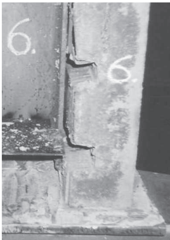
Fig. 2.8. General deformations of the analysed experimental model of the shear connection (photo Nawrot, Kucharczuk, 2004)
