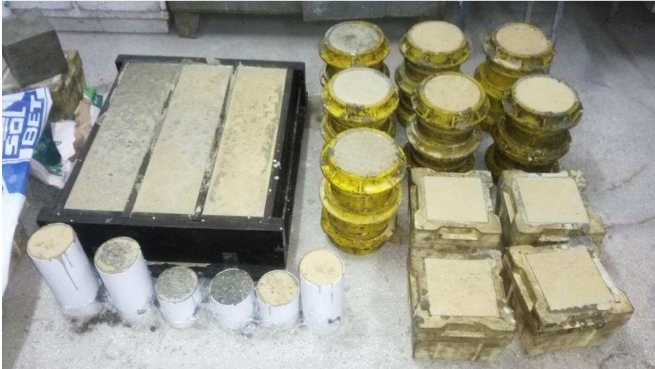
Fig. 1.2. Example of preparation of laboratory samples for one set of mixtures
