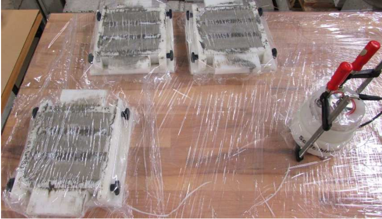
Fig. 8.6. Specimens – 9 prisms of 40 \times 40 \times 160 mm and 1 Vicat's ring
