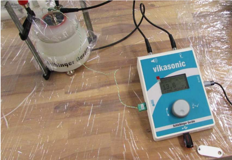
Fig. 8.7. Measurement using the ultrasonic device during setting and early hardening
