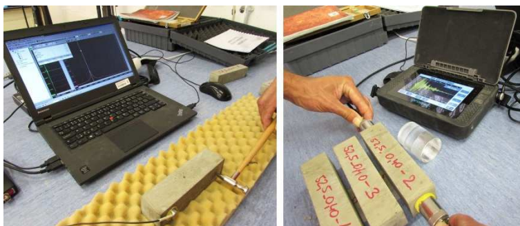
Fig. 8.8. Measurement using the resonance method (left) and the ultrasonic pulse velocity test (right)
