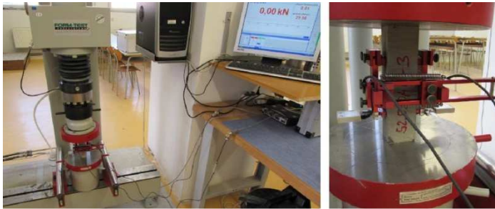
Fig. 8.9. Measurement of the static modulus of elasticity (left) and a detailed view of the strain transducers (right)
