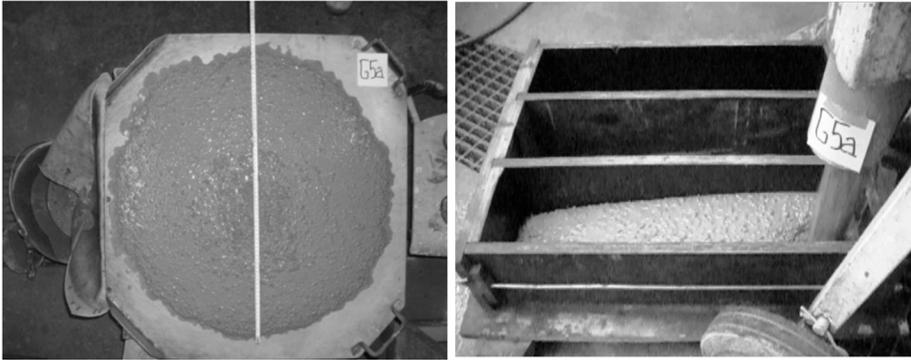
**Fig. 9.2.** Slump-flow test and forming SFRHPSCC beam C4 600x150x150 mm
