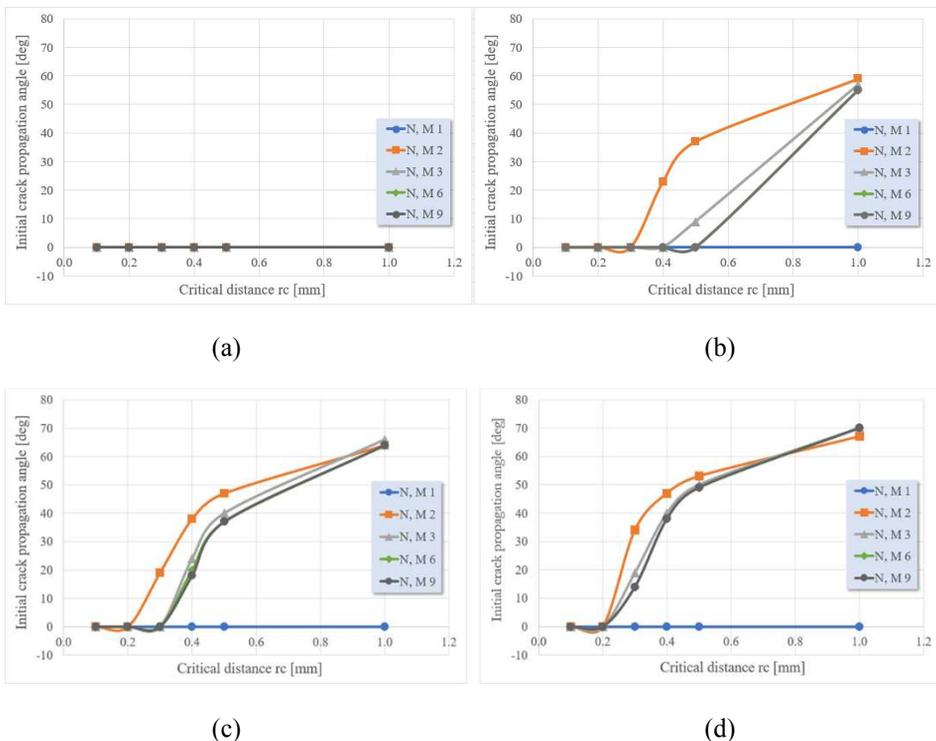
**Fig. 12.3.** How the initial crack propagation angle depends on the critical distance where the generalized (multi-parameter) MTS criterion (considering 1, 2, 3, 6 and 9 initial terms of the WE) is applied: (a) CT specimen,  $W = 30$  mm, (b) DCB specimen,  $W = 60$  mm, (c) DCB specimen,  $W = 90$  mm, (d) DCB specimen,  $W = 150$  mm
