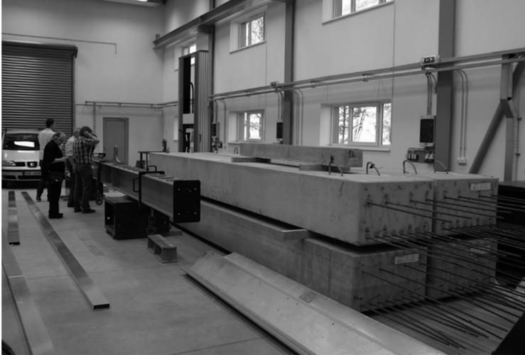
**Fig. 2.1.** Prestressed reinforced concrete beams.
