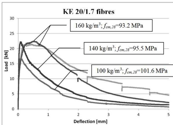
**Fig. 9.9.** Load-deflection curves and compressive strength tests for SFRSCC with KE 20/1.7 fibres (100 - 140 - 160 kg/m<sup>3</sup>)
