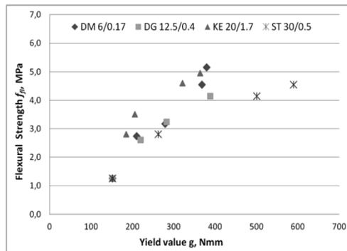
**Fig. 9.11.** Flexural strength  $f_{fl}$  - yield value  $g$  curves for SFRSCC with steel fibres
