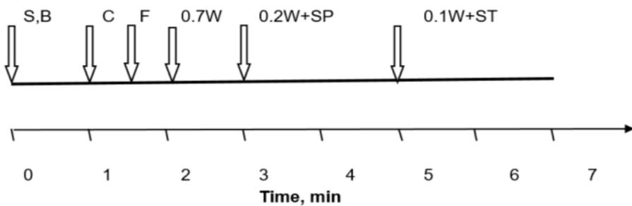
**Fig. 9.2.** Mixing procedure of SFRSCC
