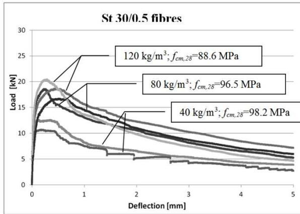
**Fig. 9.10.** Load-deflection curves and compressive strength tests for SFRSCC with ST 30/0.5 fibres (40 - 80 - 120 kg/m<sup>3</sup>)
