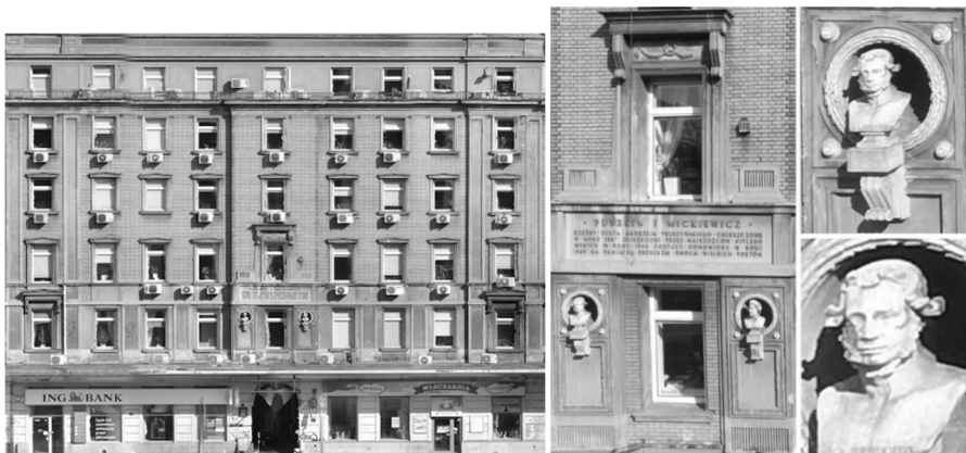
Fig. 7.5. Example of elevation orthophoto generated on UAV images, and enlargements
