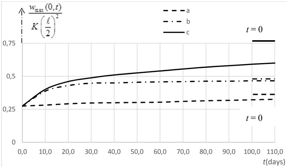
**Fig. 6.9.** Time dependent change of deflections in the middle of the plate strip, when creep occurs only in the material of plate (curve *a*), when creep occurs only in the material of subgrade (curve *b*), and when creep occurs in the material of plate, as well in that of subgrade simultaneously (curve *c*).
