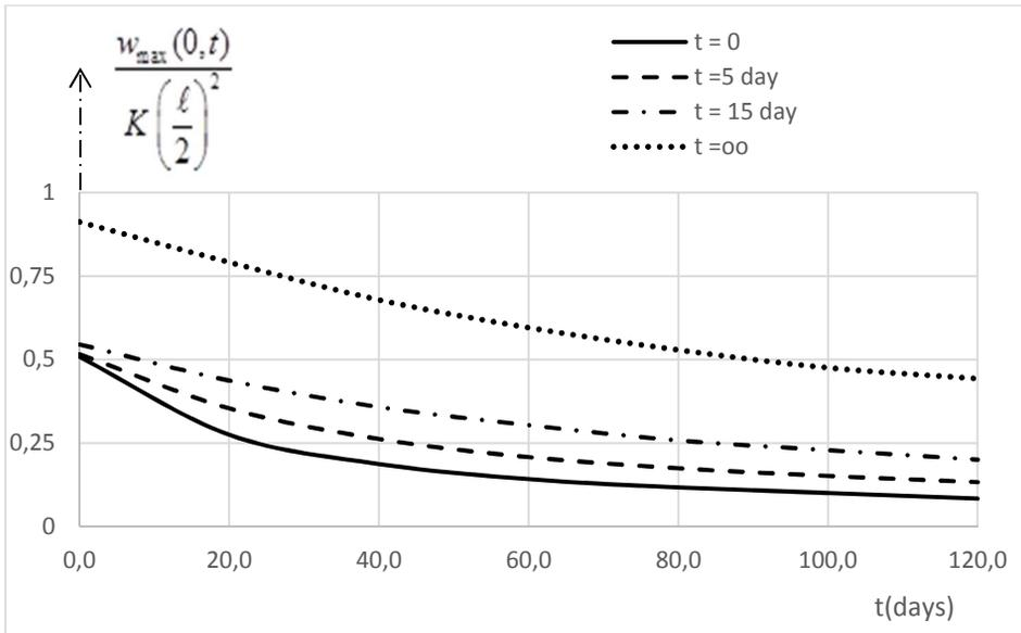
**Fig. 6.11.** Change of maximum deflections of the plate strip in time  $t$  at simultaneous creep of plate and of subgrade, when flexibility of the strip is gradually obtaining the following values:  $k = 0, 20, 40, \dots, 120$ .
