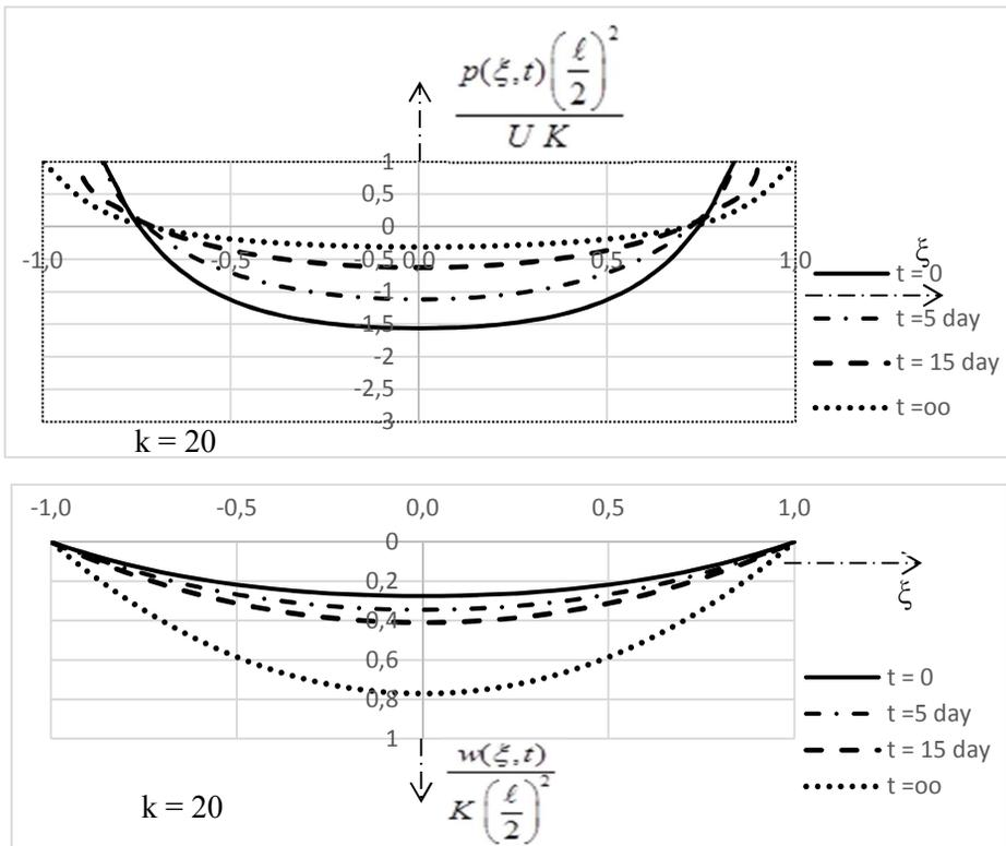
**Fig. 6.7.** Graphs of contact stresses  $p(\xi, t)$  and of deflections  $w(\xi, t)$  corresponding to the different instances  $t$  due to continuous temperature field according to Fig. 6.6, when the simultaneous creep of plate and of half-space occurs.
