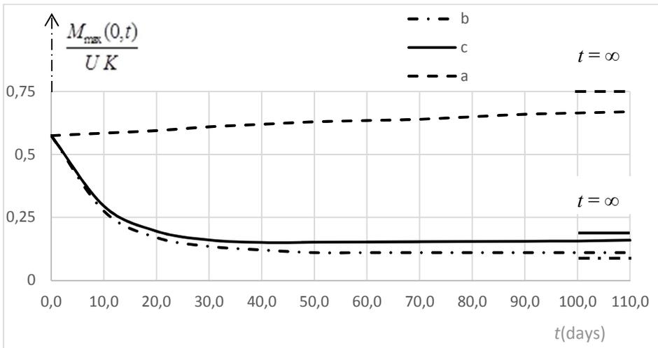
**Fig. 6.10.** Time dependent change of bending moments in the middle of the plate strip, when creep occurs only in the material of plate (curve *a*), when creep occurs only in the material of subgrade (curve *b*), and when creep occurs in the material of plate, as well as in that of subgrade simultaneously (curve *c*).
