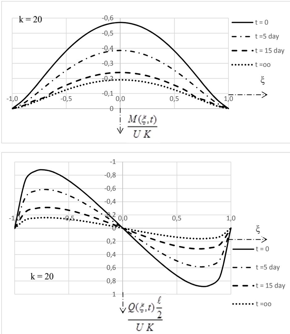
**Fig. 6.8.** Graphs of bending moments  $M(\xi, t)$  and of shear forces  $Q(\xi, t)$  in different instances  $t$  due to temperature field according to Fig. 6.6, when creep of material both of the plate and that of the subgrade occur simultaneously.
