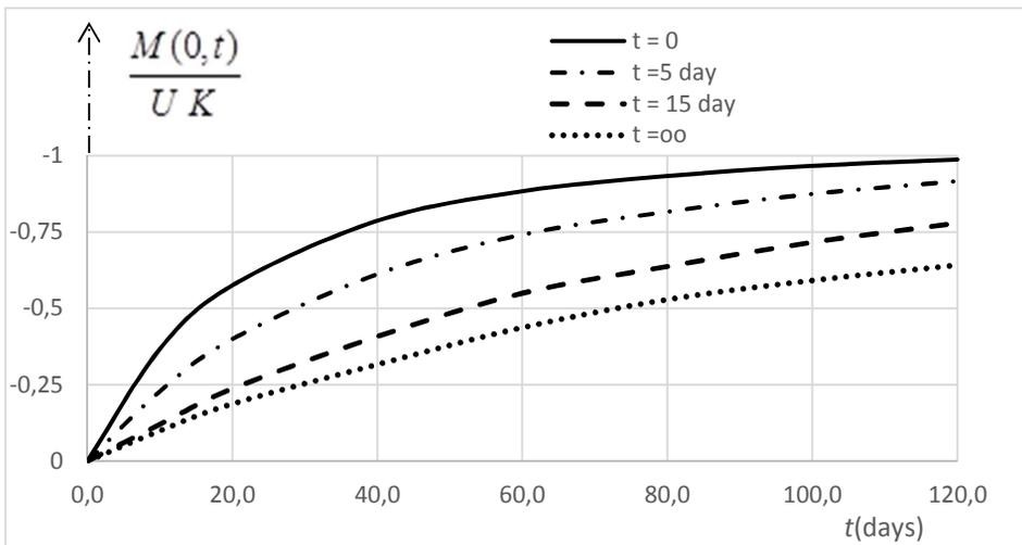
**Fig. 6.12.** Change of maximum bending moments of the plate strip in time  $t$  at simultaneous creep of plate and of subgrade, when flexibility of the strip is gradually obtaining the following values:  $k = 0, 20, 40, \dots, 120$ .
