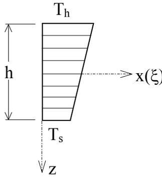
Fig. 6.4. Linear temperature gradient along the plate thickness  $h$
