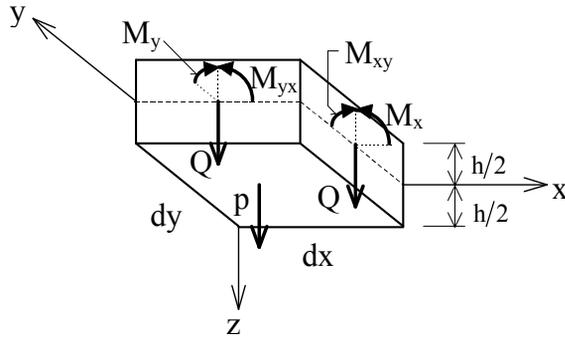
**Fig. 6.3.** Differential element of the plate strip placed on the half-space with a volume of  $dV = dx dy h$  under the actions of contact stresses  $p$  and the section quantities  $M_x, M_y, M_{xy}, Q_x, Q_y$ .
