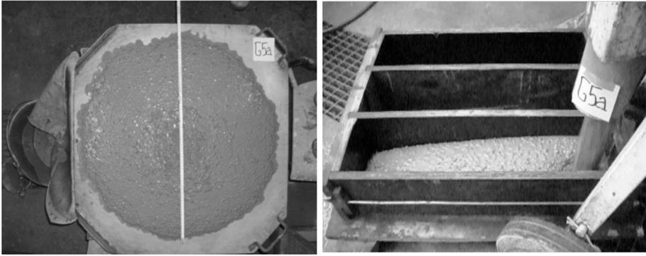
**Fig. 9.2.** Slump-flow test and forming SFRHPSCC beam C4 600x150x150 mm
