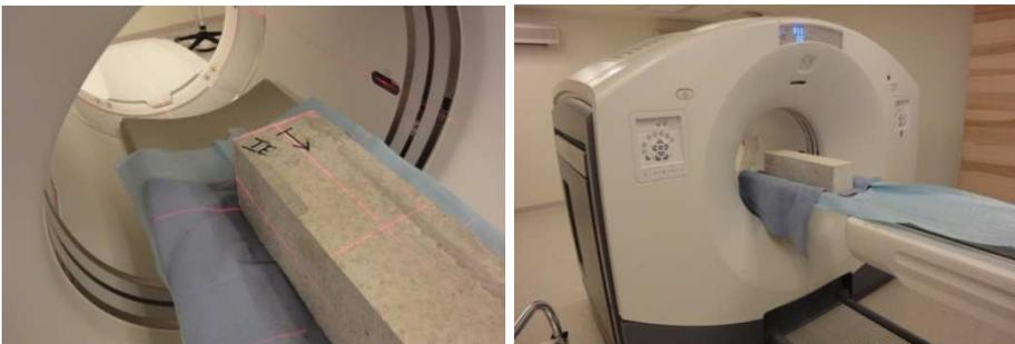
**Fig. 9.4.** The CT scanner applied for this research was equipped with 64 rows of detectors, and the thickness of a series of reconstructed native CT scan was 0.625 mm
