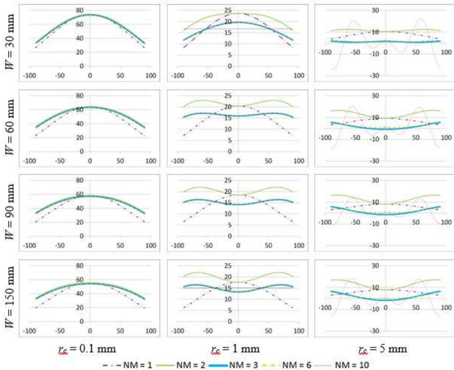
**Fig. 12.2.** Dependence of the tangential stress distribution (vertical axes in [MPa]) ahead of the crack tip on the angle  $\theta$  between  $-90^\circ$  and  $90^\circ$  (horizontal axes) for various critical distances  $r_c = 0.1, 1$  and  $5$  mm approximated via WE assuming 1, 2, 3, 6 and 10 initial higher-order terms. Each row corresponds to the cracked specimen with different width:  $W = 30$  (CT),  $W = 60, 90$  and  $150$  mm (DCB)
