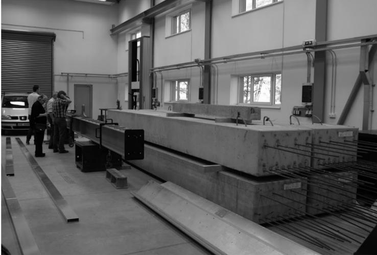
**Fig. 2.1.** Prestressed reinforced concrete beams.
