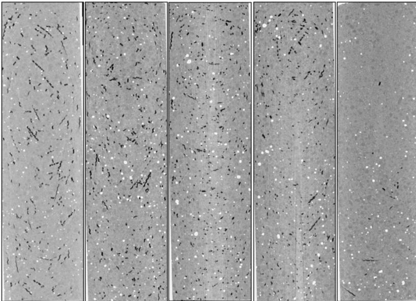
**Fig. 9.13.** X-ray 2D images of SFRSCC beams sections with ST 30x0.5 fibres; located at 1 - 3 - 7 - 10 - 14 cm from its down of beam
