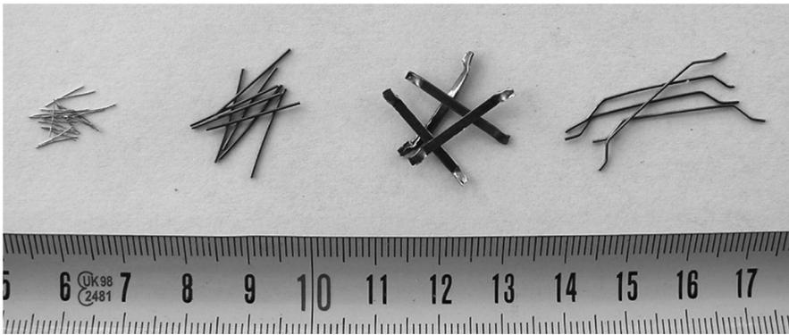
**Fig. 9.1.** Type of steel fibres used in the study: DM 6/0.17 ; DG 12.5/0.4 ; KE 20/1.7 ; ST 30/0.5
