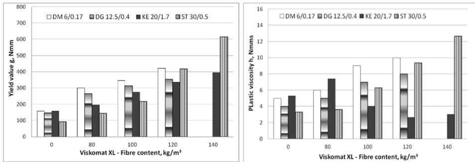
Fig. 9.5. Influence of steel fibres kind and volume on rheological properties of SFRSCC according Viskomat XL research; a) yield value g; b) plastic viscosity h
