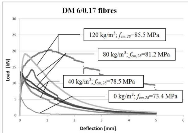
Fig. 9.7. Load-deflection curves and compressive strength tests for SFRSCC with DM 6/0.17 fibres (0 - 40 - 80 - 120 kg/m<sup>3</sup>)
