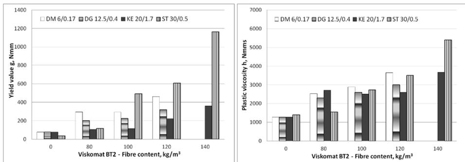
**Fig. 9.4.** Effect of steel fibres type and volume on rheological properties of SFRSCC according Viskomat BT2 research; a) - yield value  $g$ ; b) - plastic viscosity  $h$
