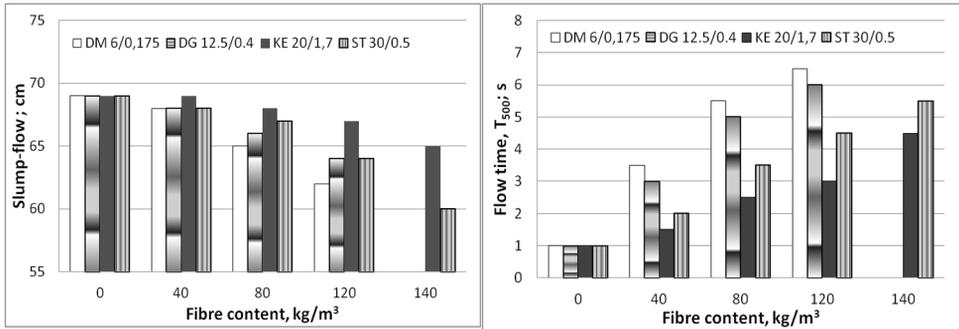
**Fig. 9.3.** Effect of steel fibres type and volume on slump-flow properties of SFRSCC; a) - slump-flow  $SF$  value; b) - flow time  $T_{500}$  value
