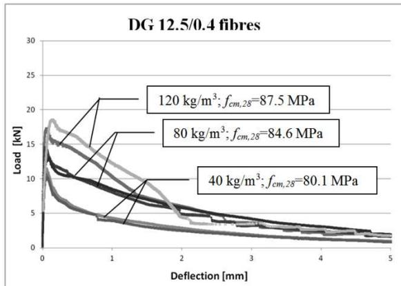
**Fig. 9.8.** Load-deflection curves and compressive strength tests for SFRSCC with DG 12.5/0.4 fibres (40 - 80 - 120 kg/m3)
